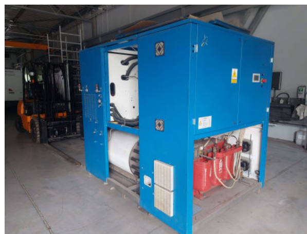
Elektrolizer PEM 100 kW, 20 Nm 3 /h, 4 bary
